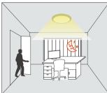
With movement and insufficient ambient lux level, the light is triggered on 100% by the detector.
